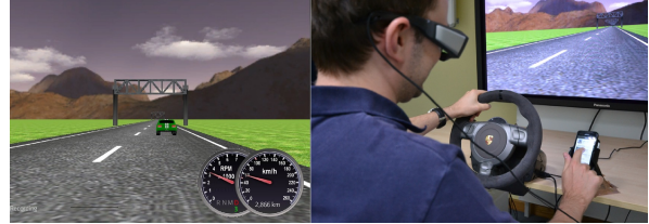
Figure 1: Experimental task (left) and set-up (right): In each of the three trials, participants were to follow the lead car while they interacted with a docked smartphone in the driving simulator.
