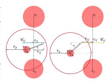
Fig. 7: Circle classification tests. The left schema represents the occlusion test while the right represents the intersection test.  $\gamma$  is the distance that is compared to the radius of  $a_k$ 's SAS sphere.
