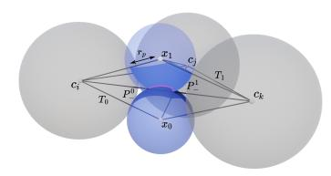
Fig. 6: Illustration of the concave patches  $P_-$ . We can notice two intersecting concave patches  $P_-$  and their respective tetrahedra. As illustrated, two  $P_-$ 's spheres can intersect resulting in a hole in the surface.
