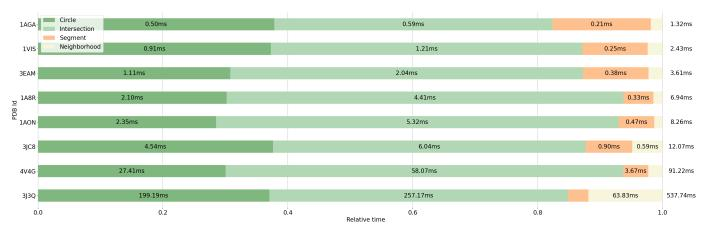
Fig. 14: Detailed GPU benchmarks of the full surface computation with a probe radius  $r_p = 1.4$  Å on a subset of our test dataset. As illustrated, respective relative computation times are correlated to the molecule geometry influencing stage complexity. A similar analysis performed for Krone et al. [28]'s method is given as supplemental material.
