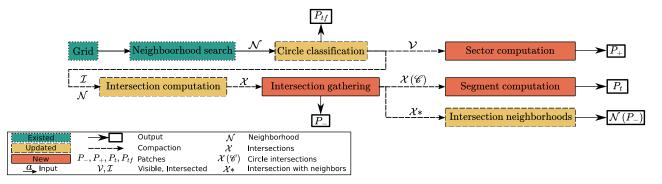
Fig. 8: Illustration of the computation pipeline giving the geometry of the complete SES. The schema also emphasizes the modification we made to the state-of-the-art SES computation method on GPUs [28].
