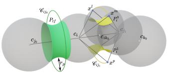
Fig. 5: Illustration of toroidal patches  $P_t$  and  $P_{tf}$ . On the illustration, we can see three toroidal patches and their corresponding SAS structures. Both kinds of patches are defined by the SAS circle coming from the intersection of the SAS spheres of their atoms, while  $P_t$  are also bounded by their corresponding intersections. In green: a complete circle patch  $P_{tf}$  with its circle. In yellow: two segments patches  $P_t$  on the same circle.
