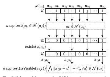
Fig. 12: Schema of the cooperative SAS intersection process used in algorithm 1. The warp is refining intersections that must be computed by iteratively modifying the bit mask  $\mathcal{K}$ . Dotted lines: intra-warp operation processed in parallel with all warp's threads but iteratively for each entry in  $\mathcal{K}$  set to one.
