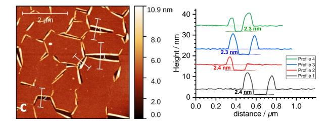
**Figure 4.** AFM images of pristine (a), plasma-treated (b) and ferrocene-grafted (c)  $MoS_2$  deposited on SiO<sub>2</sub>/Si. (Right) Corresponding cross-section profiles taken along the lines in the left images.
