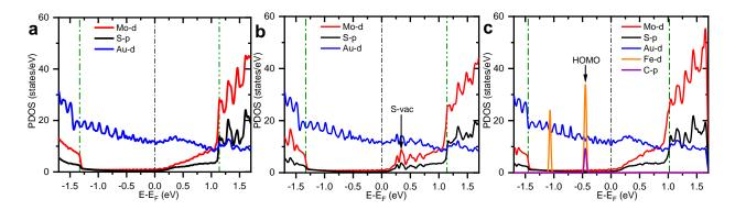
**Figure 11.** PDOS for (a) pristine MoS<sub>2</sub>/Au, (b) defective MoS<sub>2</sub>/Au and (c) ferrocene-grafted MoS<sub>2</sub>/Au. Black dashed line refers to the Fermi level and green dashed lines indicate valence band maximum (VBM) and conduction band minimum (CBM) of MoS<sub>2</sub>.
