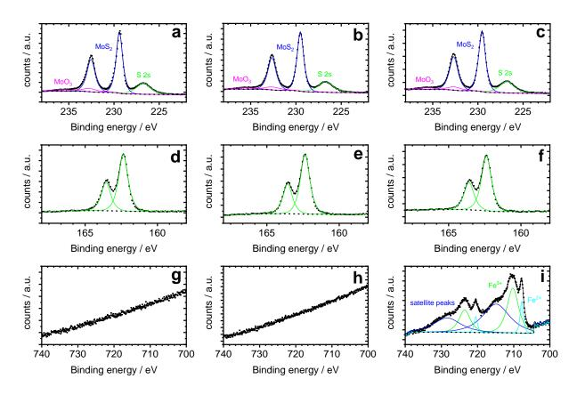
**Figure 3.** High-resolution XPS spectra for the Mo 3d (a-c), S 2p (d-f) and Fe 2p (g-i) peaks of pristine (a, d, g), plasma-treated (b, e, h) and ferrocene-grafted (c, f, i) MoS<sub>2</sub> deposited on SiO<sub>2</sub>/Si. Experimental data and fitting envelopes are represented by black dotted and solid lines, respectively. The colored lines are fitted curves using Gaussian–Lorentzian mixed peaks corresponding to different components.
