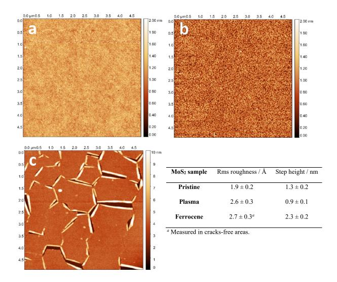
**Figure S6.** AFM images (5 x 5  $\mu$ m<sup>2</sup>) of pristine (a), plasma-treated (b) and ferrocene-grafted (c) MoS<sub>2</sub> deposited on SiO<sub>2</sub>/Si. (Bottom right) Root-mean-square roughness and step height determined by AFM (see Fig. 4 in the main text).
