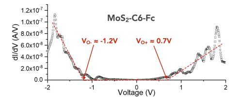
**Figure S12**. First derivative  $\partial I/\partial V - V$  (numerical derivation from the mean  $\overline{I} - V$  curve) of the ferrocene-grafted MoS<sub>2</sub> sample.
