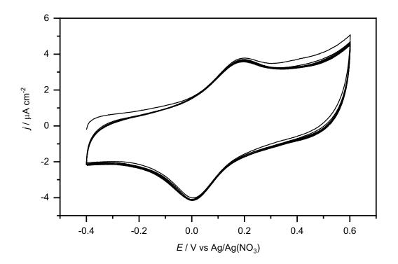
**Figure S8.** Cyclic voltammograms at 100 mV s<sup>-1</sup> of defective  $MoS_2$ -coated  $SiO_x /p^{++}Si(100)$  surface after immersion for 24 h into an acetone solution containing (ferrocenyl)hexanethiol at 1 mM over the course of 10 successive scans. Electrolyte:  $CH_3CN + 0.1M Bu_4NClO_4$ .
