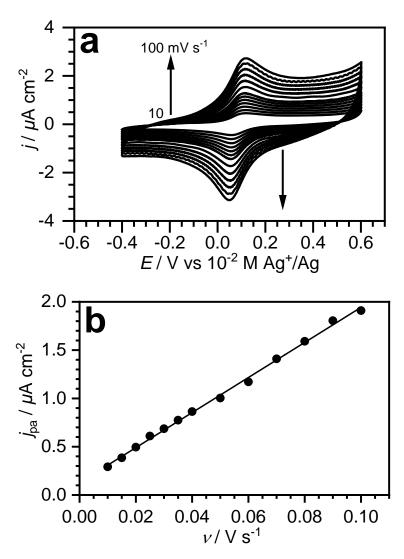
**Figure 5.** a) Cyclic voltammograms at different scan rates between 10 and 100 mV s<sup>-1</sup> of ferrocene-functionalized MoS<sub>2</sub> deposited on SiO<sub>x</sub>/Si in CH<sub>3</sub>CN + 0.1 M Bu<sub>4</sub>NClO<sub>4</sub>. b) Corresponding plot of the anodic peak current density  $j_{pa}$  versus the potential scan rate *v*.
