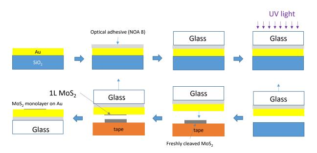
Figure S2. Preparation of MoS<sub>2</sub> monolayer-coated Au surfaces.
