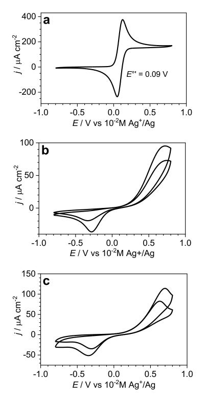
**Figure S7.** Cyclic voltammograms of ferrocene (1 mM) at a 1 mm-diameter platinum electrode at 80 mV s<sup>-1</sup> (a), SiO<sub>x</sub>/ $p^{++}$ Si(100) (b) and MoS<sub>2</sub>-coated SiO<sub>x</sub>/ $p^{++}$ Si(100) (c) at 20 and 40 mV
