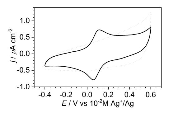
**Figure S9.** Cyclic voltammograms at 0.02 V s<sup>-1</sup> in CH<sub>3</sub>CN + 0.1 M Bu<sub>4</sub>NClO<sub>4</sub> of bare  $SiO_x/p^{++}Si(100)$  (dotted line) and defective  $MoS_2$ -coated  $SiO_x/p^{++}Si(100)$  (solid line) surfaces after immersion for 24 h into an acetone solution containing 6-(ferrocenyl)hexanethiol at 1 mM.
