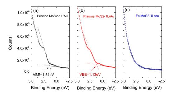
Figure S13. UPS of the (a) pristine, (b) plasma-treated and (c) ferrocene-grafted  $MoS_2$  samples near the Fermi level. The intercepts of the dashed lines are used to define the valence band edge of  $MoS_2$ .
