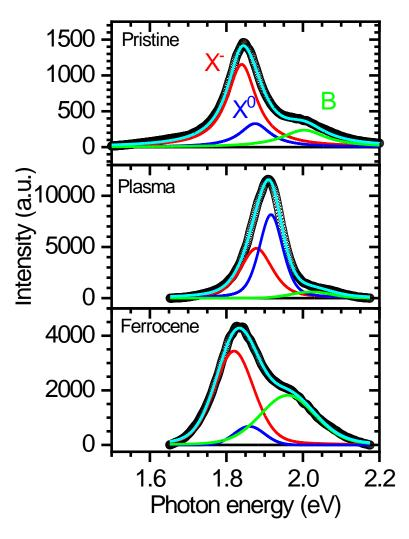
**Figure 2.** Photoluminescence spectra of pristine, plasma-treated and ferrocene-grafted MoS<sub>2</sub> deposited on SiO<sub>2</sub>/Si.
