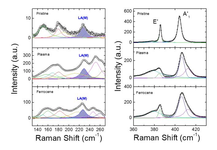
Figure S5. Fitting results of Raman spectra after background subtraction for pristine, plasmatreated and ferrocene-grafted  $MoS_2$  monolayer in the LA(M) (left) and the E' and A'<sub>1</sub> (right) regions.
