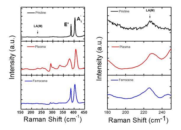
**Figure 1.** (Left) Raman spectra of pristine, plasma-treated and ferrocene-grafted MoS<sub>2</sub> deposited on SiO<sub>2</sub>/Si. (Right) Zoom on the LA(M) peak.
