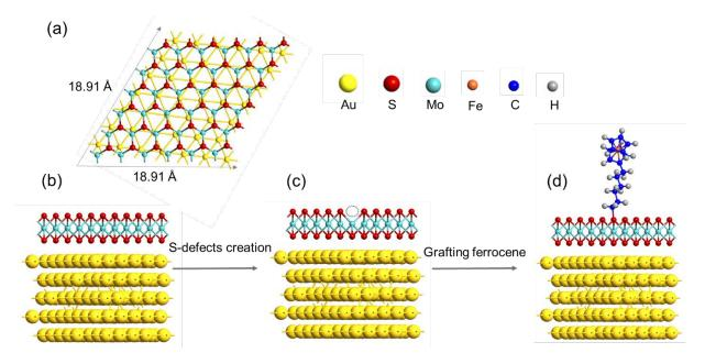
**Figure 10.** (a) Top view of the simulated supercell of the MoS<sub>2</sub>/Au interface with the Au (111) surface strained by 0.18%. A side view of the optimized (b) pristine MoS<sub>2</sub>/Au, (c) defective MoS<sub>2</sub>/Au created by removing one sulfur atom from pristine MoS<sub>2</sub>/Au, and (d) functionalized MoS<sub>2</sub>/Au created by grafting 6-(ferrocenyl)hexanethiol on defective MoS<sub>2</sub>/Au.
