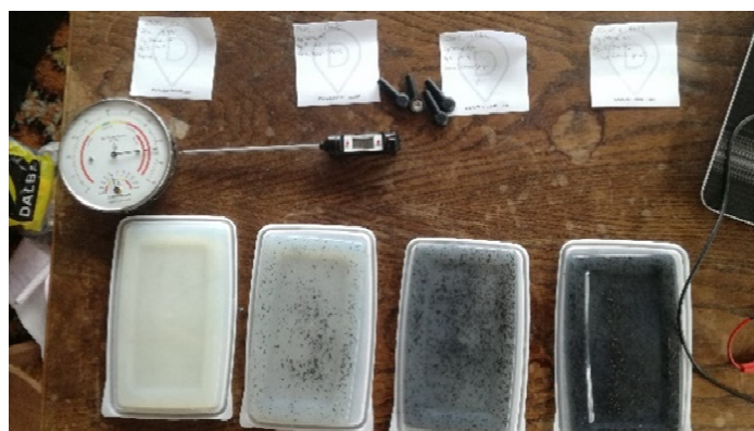
Figure 2. Gradient of 4 AA phantom of different graphite concentration (0, 12, 24 and 36 g/L).
