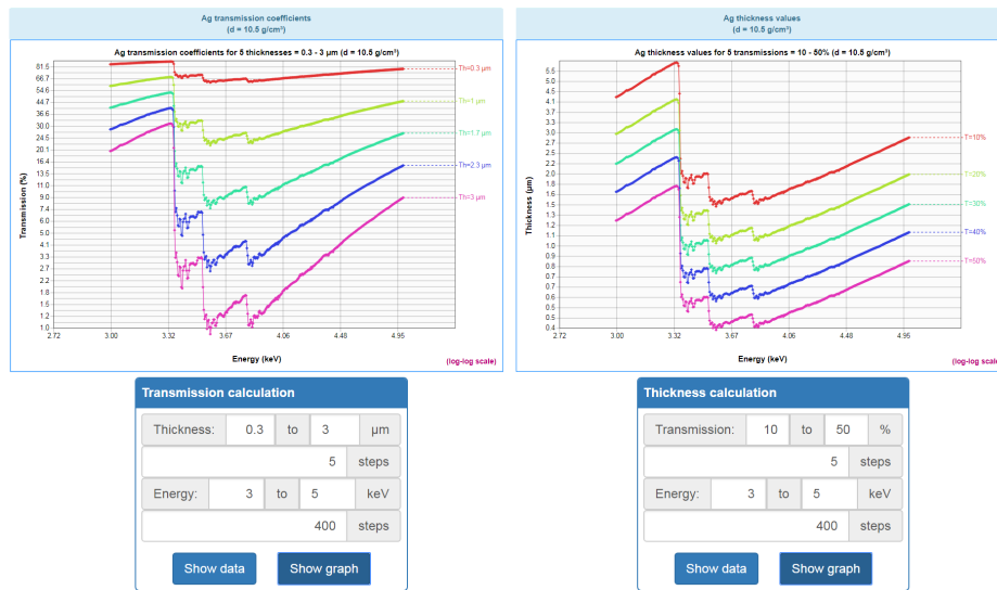
Figure 5: Example of the tools available at ( http://www.nucleide.org/Laraweb/Mu/ ) on Ag close to the L absorption edges.
