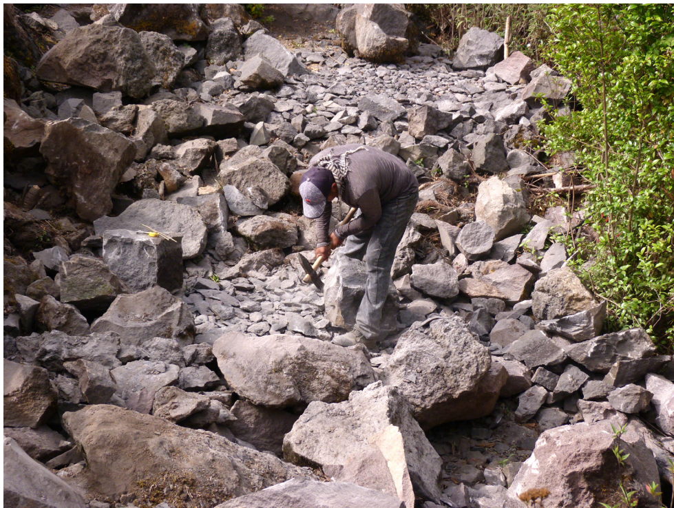
Figure 18. El Metate “El Cerro”: workshops on terraces from zone C exploited today by Nicolás Vidales, here shaping a metate roughout with an iron pick.
