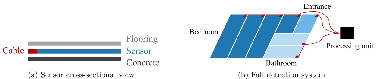
Figure 3: (a) Sensor view. A roll of sensor can be installed directly onto the concrete and covered by the flooring. (b) In this installation example, there are three areas (bathroom, bedroom and entrance) and all signals are sent to a processing unit.
