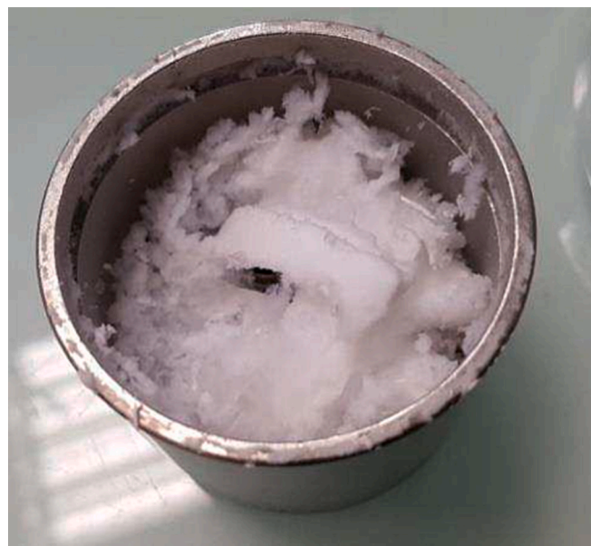
Fig. 5. Powder obtained with experiment 3 performed at 150 bar, 40 °C, u = 2.6 m·s -1 , X = 21.6 (mass ratio), and C° = 0.3 g·(kg solvent ) -1 .
