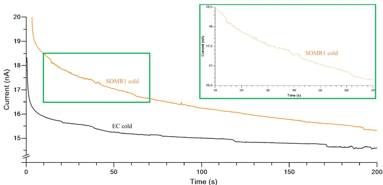
**Fig. 5.**  $i-t$  curves recorded on a 7  $\mu\text{m}$ -diameter CF UME at +0.8 V vs Ag/AgCl in 2 mL of 50 mM  $\text{K}_4\text{Fe}(\text{CN})_6$  0.1 M PBS at pH 7.4 under an inert atmosphere at cold temperatures, in the presence of  $\sim 10^9$  cells of EC (black) and SOMR1 (orange).
