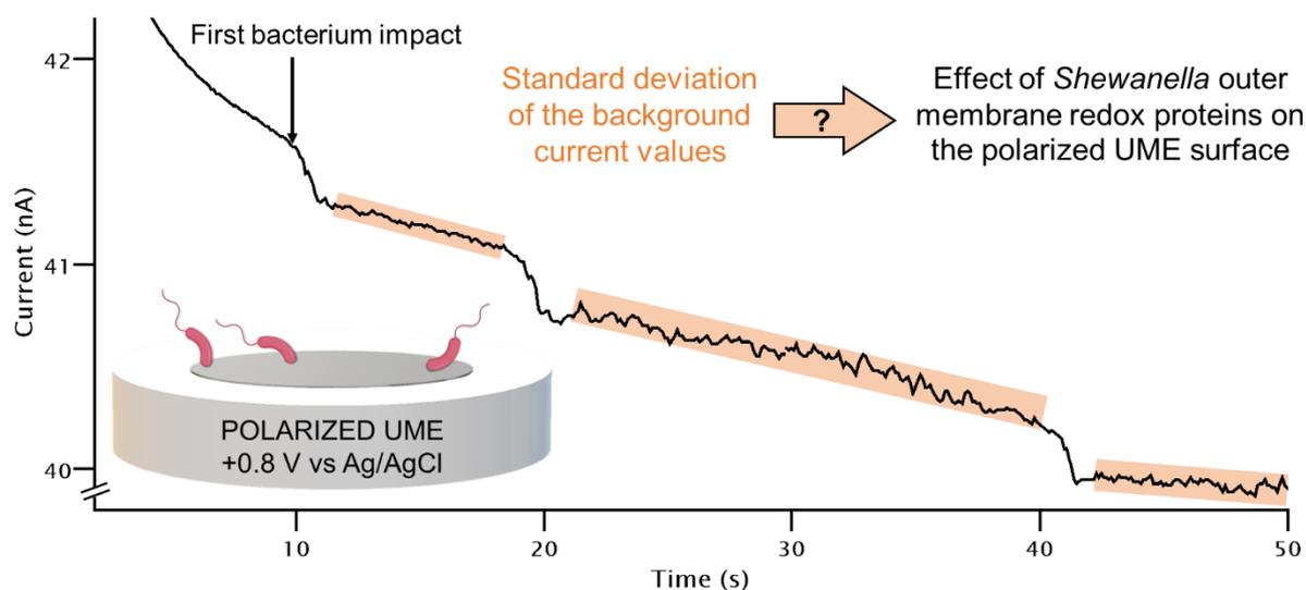
**Fig. 2.** Analysis of the current fluctuations between single blocking impact events in the  $i-t$  curve recorded in ferrocyanide aqueous solution and related to the outer membrane redox proteins involved in the bacterial cells' adhesion on the polarized UME surface.
