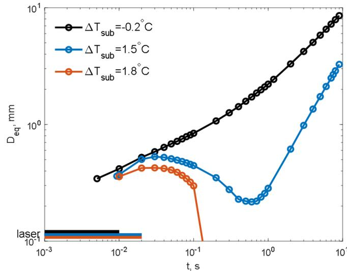
**Fig. 7** Calculated equivalent diameter of the bubble versus time. The effect of subcooling on the bubble growth. Simulation results.  $P = 600$  mbar,  $q = 0.5$  W/cm<sup>2</sup>,  $t_{wait} = 1$  s, laser pulse 10 ms (top curve) and 20 ms (middle and bottom curves).
