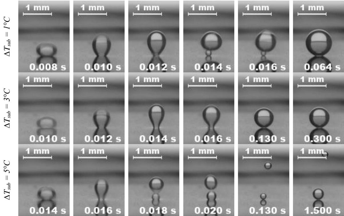
**Fig. 4** The effect of subcooling  $\Delta T_{sub}$  on bubble nucleation and stabilization.  $P = 600$  mbar,  $q = 0.5$  W/cm<sup>2</sup>,  $t_{wait} = 1$  s, laser pulse 10 ms (top row) and 20 ms (middle and bottom rows). The time indicated at each image is counted from the laser pulse start. The first image in each row shows the first bubble observed after nucleation.
