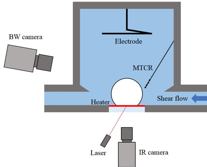
**Fig. 1** Scheme of the RUBI boiling cell.
