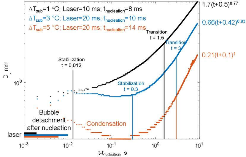
**Fig. 6** Horizontal diameter of the attached bubble versus time. The effect of subcooling on the bubble growth for several subcooling temperatures. The text “laser” and color bars show the period when the laser is activated. Power laws represent the typical bubble growth for the third stage.
