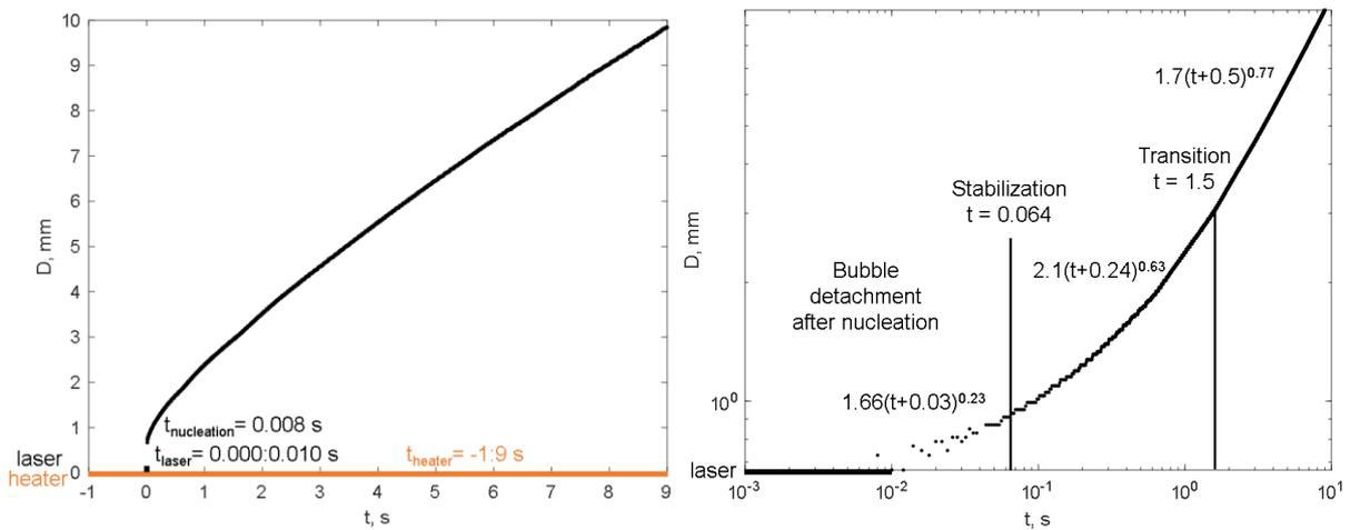
**Fig. 5** Horizontal bubble diameter evolution in time for  $P = 600$  mbar,  $q = 0.5$  W/cm<sup>2</sup>, and  $\Delta T_{sub} = 1^\circ\text{C}$  **a)** linear scale and **b)** logarithmic scale. Color text “laser” and “heater” and color bars show the period when the laser and heater are activated. Power laws show the typical bubble growth ones for different stages.
