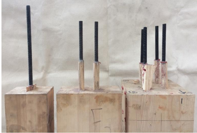
Fig. 7. Failure of specimens
