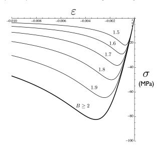
**Figure 12.** Response of proposed anisotropic damage model in equi-biaxial compression for different values of bicompression parameter *B* (dashed line: initial anisotropic damage model, thick line: unbounded  $R_{\nu}$  case  $B \to \infty$  or any case  $B \ge 2$ ).
