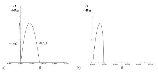
Figure 4. Response of initial anisotropic damage model a) in tension, b) in equi-biaxial tension.
