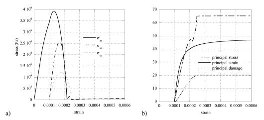
**Figure 1.** Willam's test result for initial anisotropic damage model (Ragueneau et al 2008) a) continuous stresses, b) continuous principal directions angles  $\varphi_{\sigma}$ ,  $\varphi_{\epsilon}$ ,  $\varphi_D$  (angles in degree) for stress, strain and damage tensors.
