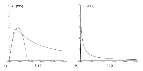
Figure 13. Response of proposed anisotropic damage model in shear (dashed curve: initial anisotropic damage model). A larger strain scale used in b).
