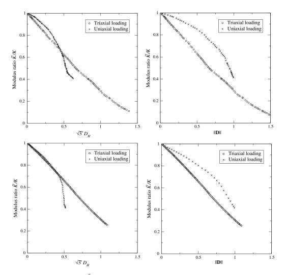
**Figure 2.** Effective bulk modulus  $\tilde{K}$  from Discrete Element computations as a function of hydrostatic damage (of  $\sqrt{3}D_H$  for comparison) and of quadratic norm  $\|\mathbf{D}\|$ . Top:  $8 \times 8 \times 8 \text{ mm}^3$  cube, bottom:  $16 \times 16 \times 16 \text{ mm}^3$  cube (from (Delaplace and Desmorat 2007)).
