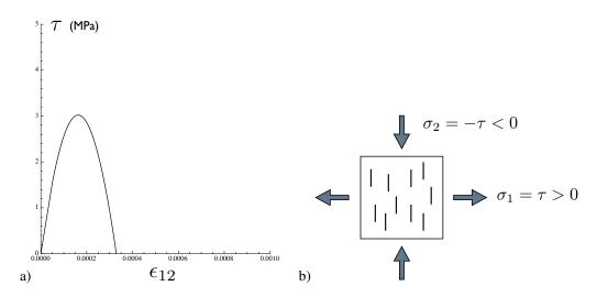
**Figure 7.** Response of initial anisotropic damage model in shear, b) Microcracking pattern corresponding to damage state  $D_1 \ge 0$ ,  $D_2 = 0$  in shear.
