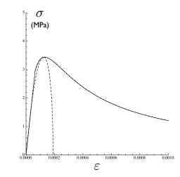
Figure 10. Response of proposed anisotropic damage model in equi-biaxial tension (dashed line: initial anisotropic damage model).
