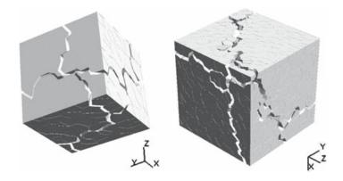
**Figure 3.** Discrete Element samples considered as Representative Volume Element (left  $8 \times 8 \times 8 \text{ mm}^3$  cube, right:  $16 \times 16 \times 16 \text{ mm}^3$  cube) and crack patterns at the end of triaxial loading (high damage level) for the two samples.
