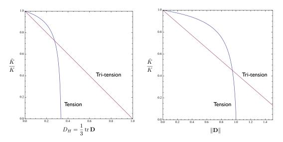
**Figure 8.** Effective bulk modulus  $\tilde{K}$  from shear-bulk coupling (23)-(30) as a function of hydrostatic damage  $D_H$  and of quadratic norm  $\|\mathbf{D}\|$  with  $\mathbf{D} = 1 - \mathbf{H}^{-2}$ .
