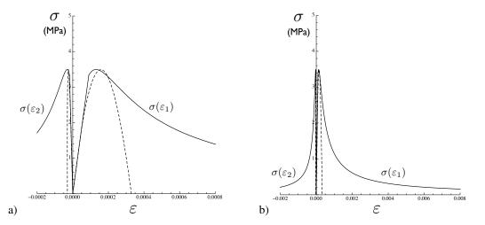
Figure 9. Response of proposed anisotropic damage model in tension (dashed line: initial anisotropic damage model). A larger strain scale used in b).
