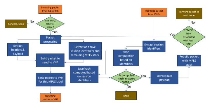
Fig. 4: Algorithm of the proxy for managing MPLS labels and VNFs
