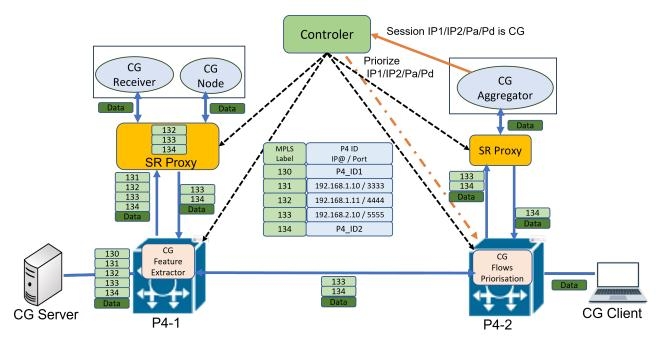
Fig. 5: Demonstrator using SR-MPLS to chain P4 and VNF micro-services for cloud gaming traffic detection and prioritization
