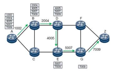
Fig. 1: Segment Routing Approach, from [11]
