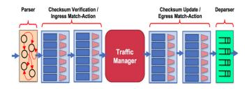
Fig. 3: Architecture of P4 programmable program, from [24]
