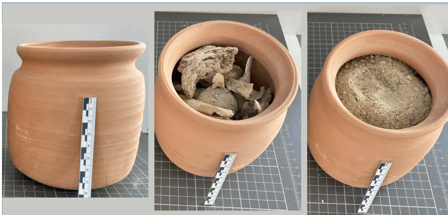
Figure 1: Photos of the artificial funerary urns, empty (left), containing bones (centre), containing bones and sand (right).
