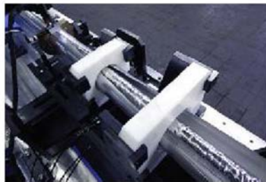
Outer tube shaping and welding process
