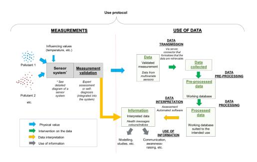
Figure 1: Typical use of a sensor system
