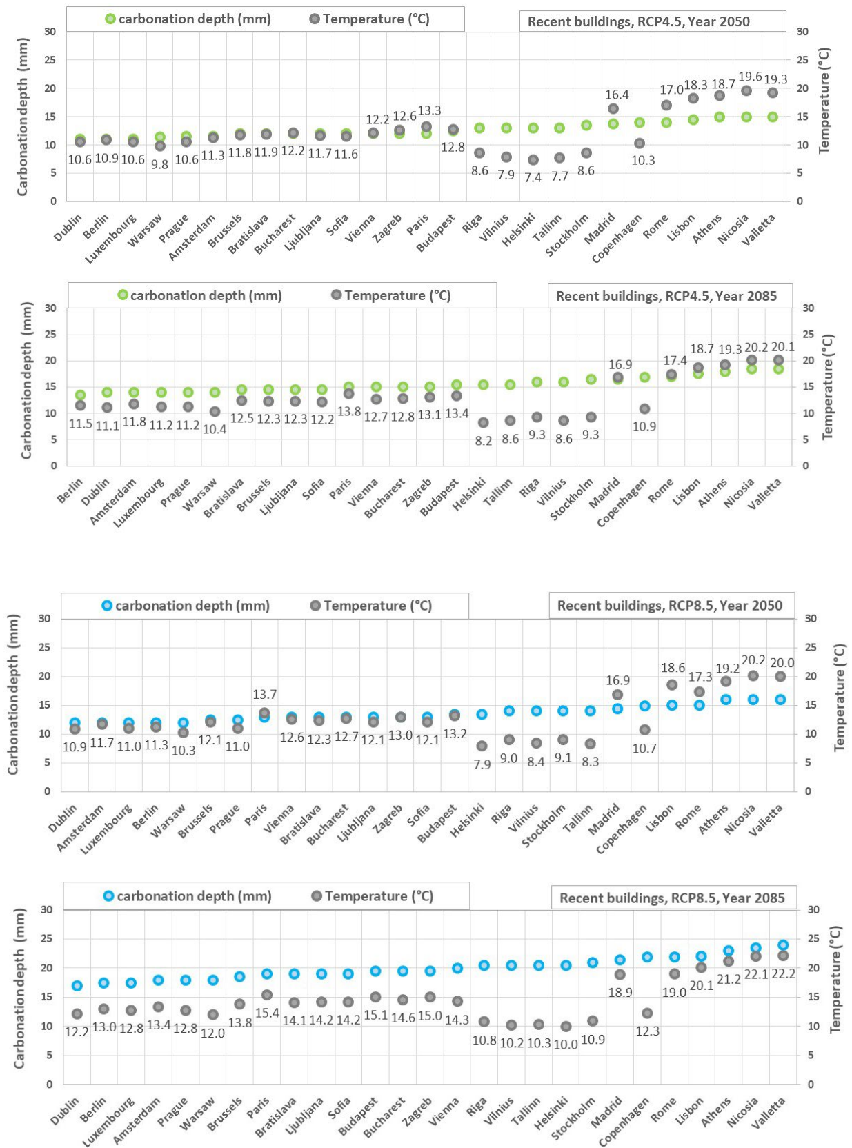
Figure 31. Absolute increase of carbonation depth in EU-27 capital cities for recent buildings , absolute temperature for a given year and temperature variation relative to the reference scenario.
