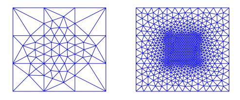
(a) Coarse grid (# Nodes =62 ) (b) Fine grid (# Nodes =895)
