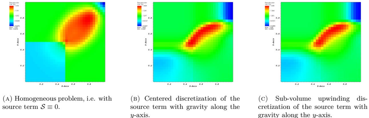
FIGURE 13. Approximate solution to a 2D Riemann problem, at final time  $T = 0.25$ . Solution obtained with no source term (left), with the centered discretization of the source term (center), and with the upwind discretization of the source term (right). For the three results shown,  $N_x = N_y = 32$ ,  $\theta = \pi/4$ ,  $C_{CFL} = .25$ .
