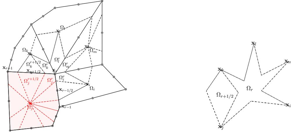
(A) Generic cell  $\Omega_j$  with its sub-cells  $\Omega_j^{dof}$  defined around nodes  $r$  and edges  $r + \frac{1}{2}$ . (B) Associated composite dual cell around node  $\mathbf{x}_r$ :  $\Omega_r = \cup_{i:r \in i} \Omega_i^r$ , and around edge  $\mathbf{x}_{r+\frac{1}{2}}$ :  $\Omega_{r+\frac{1}{2}} = \Omega_j^{r+\frac{1}{2}} \cup \Omega_k^{r+\frac{1}{2}}$ .
