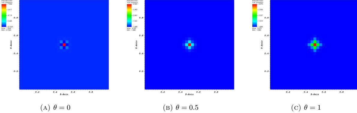
FIGURE 5. Illustration of the non-physical propagation results obtained on Cartesian mesh, with  $\theta = 0$  (left), compared to the physical propagation with  $\theta > 0$  (center:  $\theta = 0.5$ , right:  $\theta = 1$ ).
