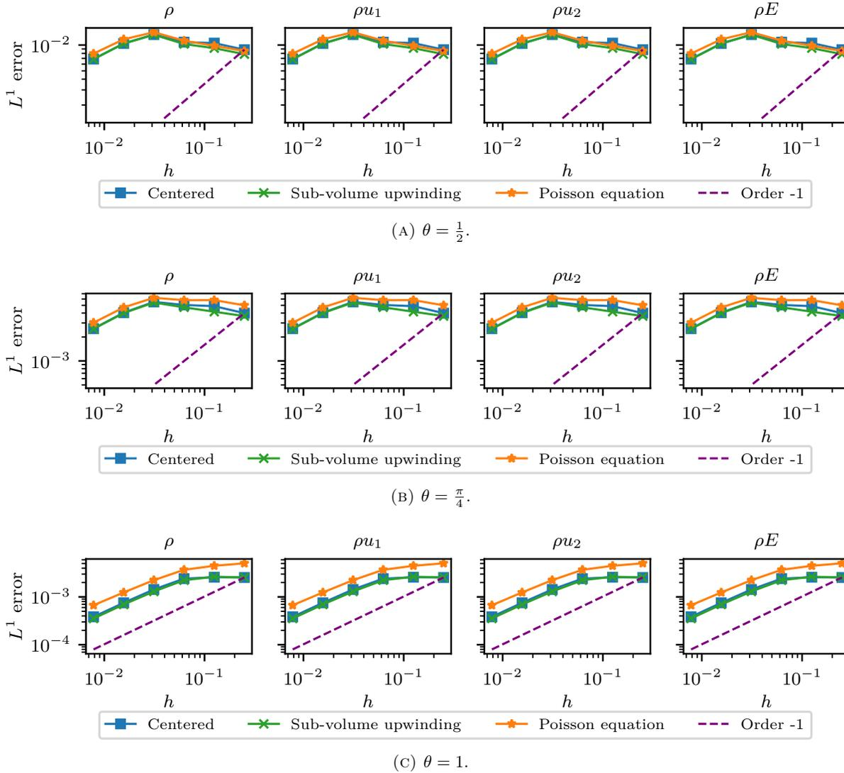
FIGURE 12.  $L^1$  error on  $\rho$  (leftmost column),  $\rho u_1$  (second column),  $\rho u_2$  (third column) and  $\rho E$  (rightmost column), for the test case 5.3 – Friction on a random mesh with  $\theta = \frac{1}{2}$  (top row),  $\theta = \frac{\pi}{4}$  (middle row), and  $\theta = 1$  (bottom row).
