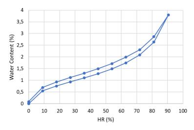
Figure 2 : Sorption isotherm of our composite of raw earth with straw
