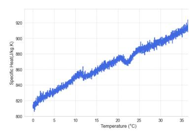
Figure 4 : Evolution of cob's specific heat depending on the temperature
