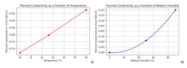
Figure 3 : Cob's thermal conductivity depending on the temperature and the Relative Humidity
