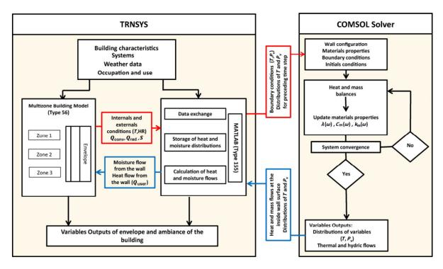
Figure 1 : HAM-BES platform operating principle [27]
