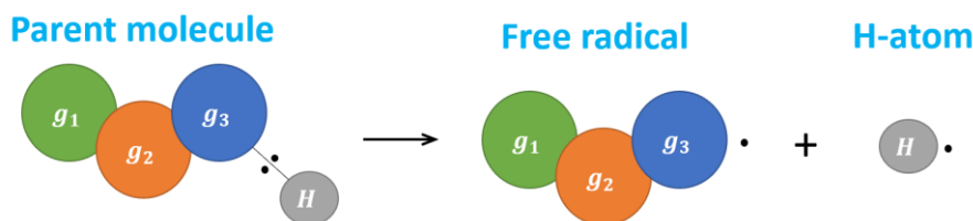
Figure 5. Generic reaction for the formation of a free radical.
