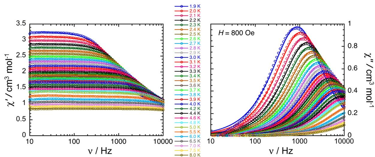
**Supplementary Figure 13.** Frequency dependence of the in-phase ( $\chi'$ ; left) and out-of-phase ( $\chi''$ ; right) components of the ac susceptibility for  $\text{Eu}\{\text{N}(\text{SiMePh}_2)_2\}_2$  (**1**) between 1.9 and 8 K for ac frequencies between 10 Hz and 10 kHz under an applied static field of 800 Oe. Solid lines represent the fits to the generalized Debye model.
