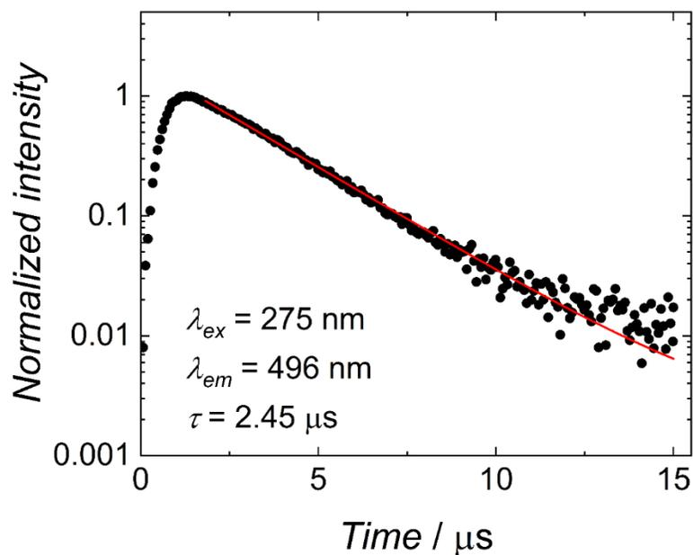
**Supplementary Figure 4.** Room-temperature emission decay (black points) and mono exponential function fit (red line) for  $\text{Eu}\{\text{N}(\text{SiMePh}_2)_2\}_2$  (**1**).
