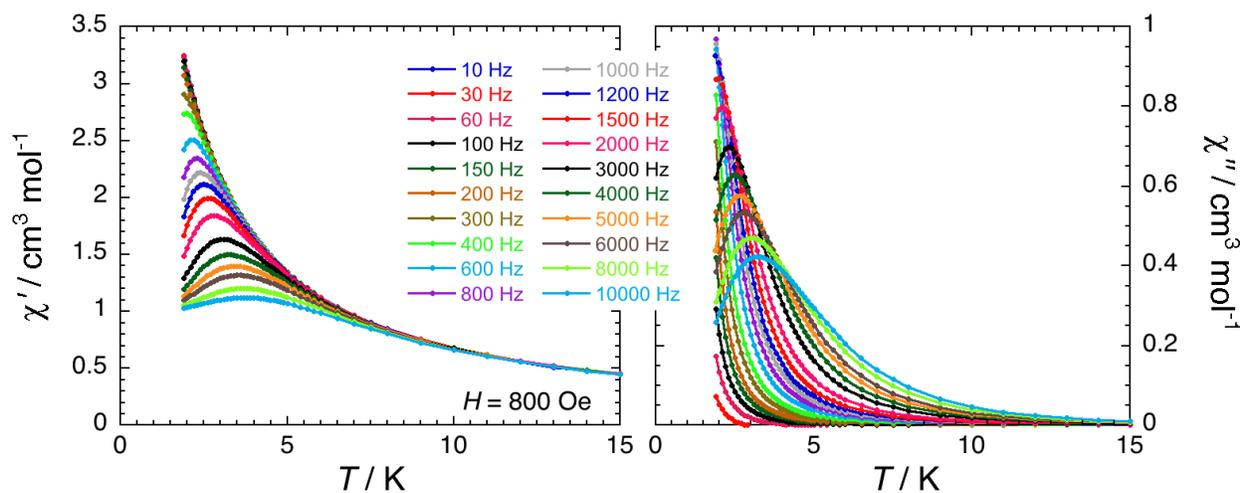
**Supplementary Figure 12.** Temperature dependence of the in-phase ( $\chi'$ ; left) and out-of-phase ( $\chi''$ ; right) components of the ac susceptibility for  $\text{Eu}\{\text{N}(\text{SiMePh}_2)_2\}_2(\mathbf{1})$  between 10 Hz and 10 kHz for the temperature range 1.9-15 K under an applied static field of 800 Oe.
