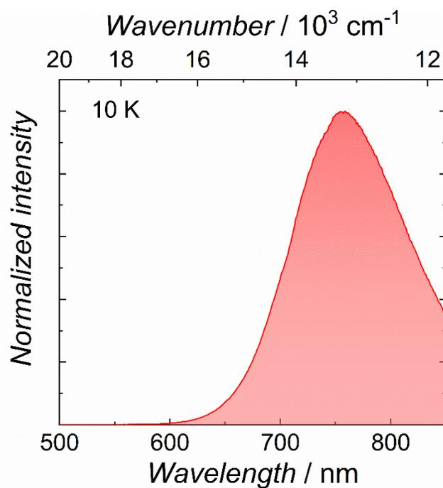
**Supplementary Figure 5.** Emission spectra for the crude oxidized product of  $\text{Eu}\{\text{N}(\text{SiMePh}_2)_2\}_2$  (**1**) obtained in  $\text{C}_6\text{H}_5\text{F}$  ( $\lambda_{\text{ex}} = 270 \text{ nm}$ ).
