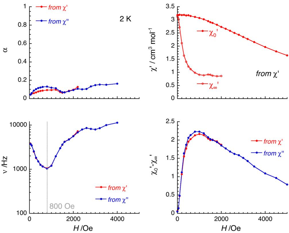
**Supplementary Figure 10.** Field dependence of the fitting parameters  $\alpha$ ,  $\nu$ ,  $\chi_0$ ,  $\chi_\infty$ , and  $\chi_0 - \chi_\infty$ , between 0 and 5 kOe at 2 K determined from the generalized Debye fit of the frequency dependence of the in-phase ( $\chi'$ ) and out-of-phase ( $\chi''$ ) components of the ac susceptibility (Supplementary Figure 9).
