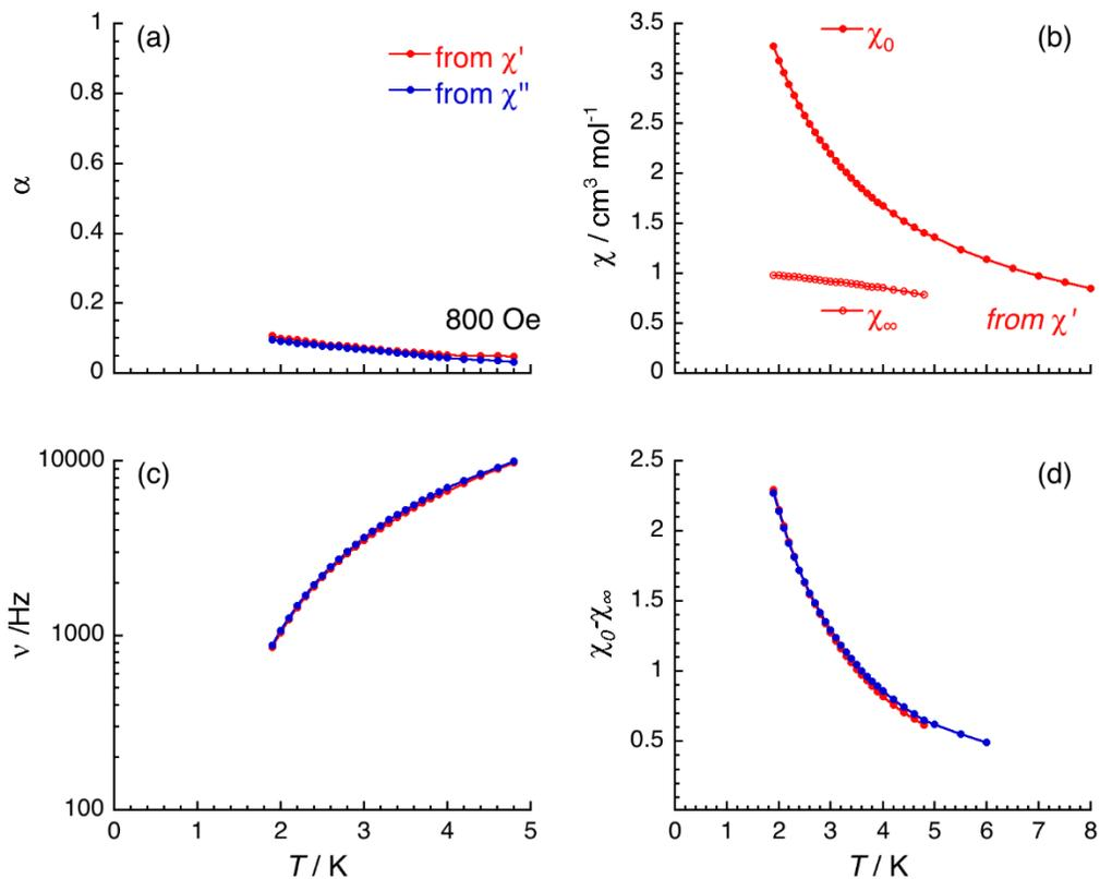
**Supplementary Figure 14.** Temperature dependence of the fitting parameters  $\alpha$ ,  $\nu$ ,  $\chi_0$ ,  $\chi_\infty$ , and  $\chi_0\chi_\infty$ , between 1.9 and 8 K under an applied static field of 800 Oe determined from the generalized Debye fits of the frequency dependence of the in-phase ( $\chi'$ ) and out-of-phase ( $\chi''$ ) components of the ac susceptibility (Supplementary Figure 13).
