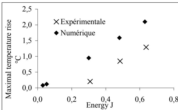
Figure 5: Maximal increase in temperature at a point of depth 2 mm as a function of the energy of the incident shot, comparison between experimental and numerical results for a shot of diameter 3 mm.
