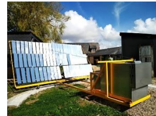
Figure 2. The Lytefire artisan solar oven used by NeoLoco (Photo: Courtesy of ©NeoLoco)
