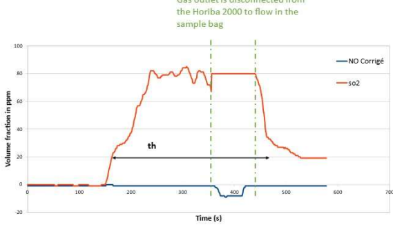
Figure 8. HORIBA readings for Flash2 test with nitrogen flowrate F_{N_2}=1.6 Nm^3/h and a biomass rate m=3 g/min
