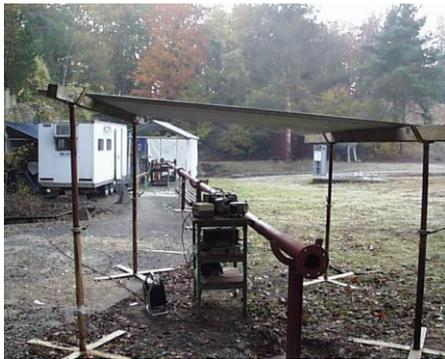
Figure 1: Flame propagation test rig
