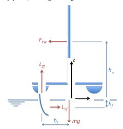
Figure 6. Schematic diagram of the boat equilibrium
