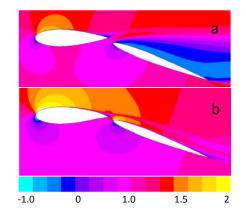
Figure 3. Contours of *U* for  $\gamma = 0^{\circ}$  (a) and  $\gamma = 10^{\circ}$  (b)
