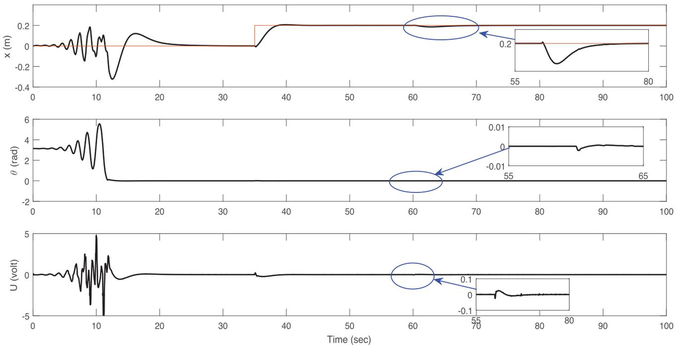
**FIGURE 15** MOPIF control result with step disturbance at  $t = 60$  s.
