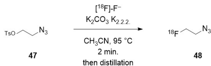
Figure 31. Synthesis of [ ^{18}\text{F} ]-fluoroethylazide 48 .
