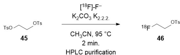
Figure 30. Synthesis of [ ^{18}\text{F} ]-fluoroethyltosylate 46 .
