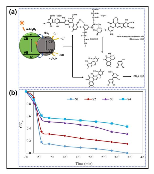
**Fig. 7** a Photocatalytic mechanism of humic acid degradation by  $\alpha$ -Fe<sub>2</sub>O<sub>3</sub>/NiS<sub>2</sub> photocatalyst. Reprinted with permission from ref. (Mohtar et al. 2021) Copyright 2021 Elsevier. **b** Cephalexin degrada-
