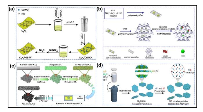
**Fig. 4** Synthesis process of **a** g-C<sub>3</sub>N<sub>4</sub>/NiS-W. Reprinted with permission from (Xue et al. 2021) Copyright 2020 Elsevier. **b** NiS-MoS<sub>2</sub>/CNTs/g-C<sub>3</sub>N<sub>4</sub> hybrid. Reprinted with permission from ref. (Zhang et al. 2018b). Copyright 2018 Elsevier. **c** NiS<sub>x</sub>-MoO<sub>2</sub>/CC. Reprinted
