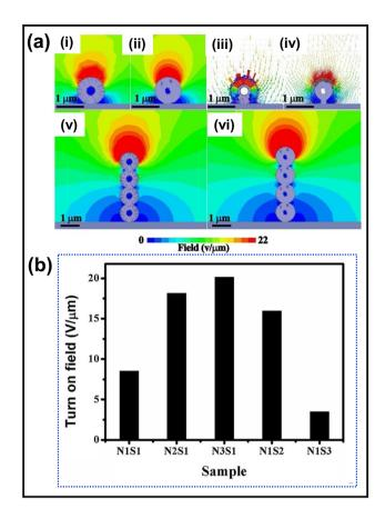
**Fig. 6 a** ANSYS simulations for output filed magnitude of nickel sulfide; individual rod-made sphere (i), particulate sphere (ii); field vectors for individual rod-made sphere (iii), particulate sphere (iv); and output filed magnitude for micro tube with rod-made sphere (v), particulate sphere (vi), and **b** turn-on fields for varying Ni to S atomic compositions (1 to 3). Reprinted with permission from ref. (Khan et al. 2021). Copyright 2021 Elsevier
