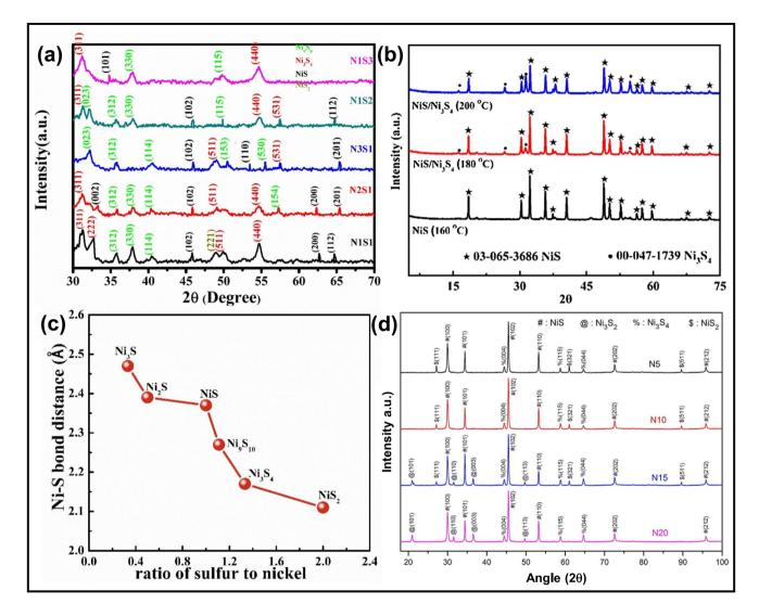
**Fig. 2** a XRD spectra of the synthesize nickel sulfides at different atomic ratios of Ni and S (1:1, 2:1, 3:1, 1:2, and 1:3). Reprinted with permission from ref. (Khan et al. 2021). Copyright 2021 Elsevier. **b** Effect of temperature (160, 180, and 200 °C) on the different phase ratios of nickel sulfides. Reprinted with permission from ref. (Gou et al. 2017). Copyright 2017 Elsevier. **c** Correlation of the S- content
