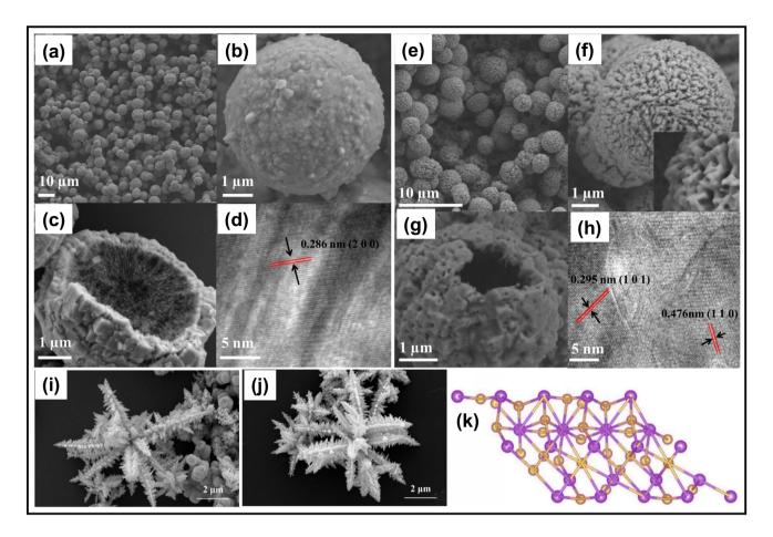
**Fig. 5** Microspheres FESEM and TEM images of NiS<sub>2</sub> (**a-d**) and NiS (**e-i**). Reprinted with permission from ref. (Luo et al. 2017). Copyright 2016 American Chemical Society. **i-j** SEM images of pure CdS and NiS/CdS (Ni/Cd ratio of 0.4) nanoflowers. Reprinted with permission from ref. (Zhang et al. 2018a). Copyright 2019 Elsevier. **k**
