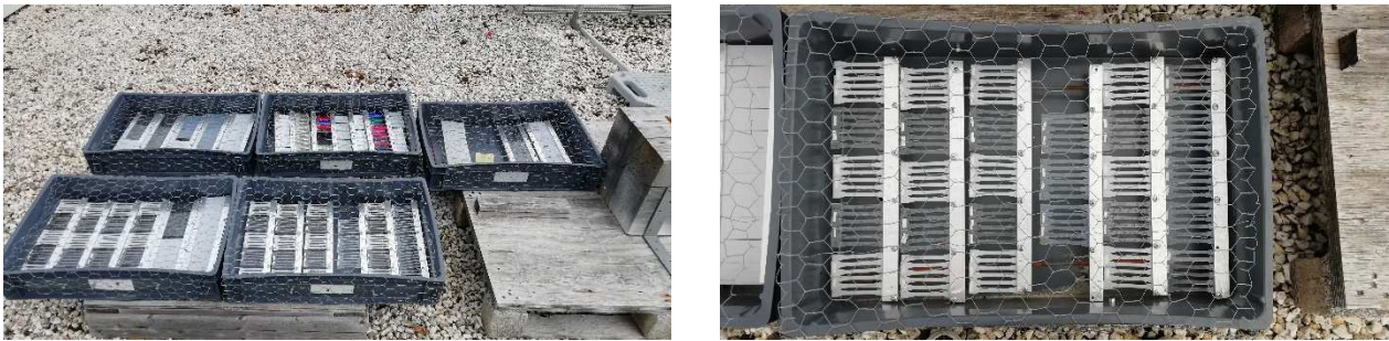
68 Figure 1 – Climatic weathering installation on the Lorient rooftop
