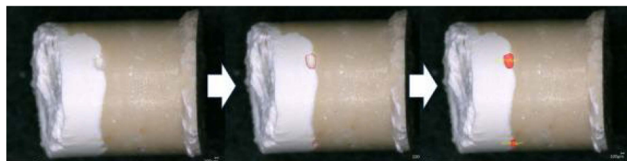
Figure 1. Digital micrographs (BD-TF) with the void quantification by using the software VHX-5000.
