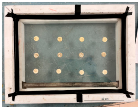
Figure 4. Teflon frame with the acetate film on top of the glass plate. The tape was used to seal the edge of the frame.
