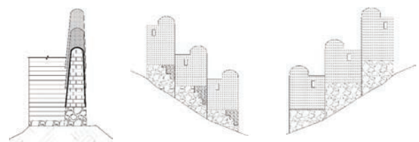
Figure 12: Drawings of The wall on adobe after restoration. © S.M. Khalili
