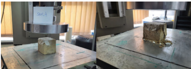
Figure 12: Adobe bricks sample 105_4 before and after compressive strength test.
