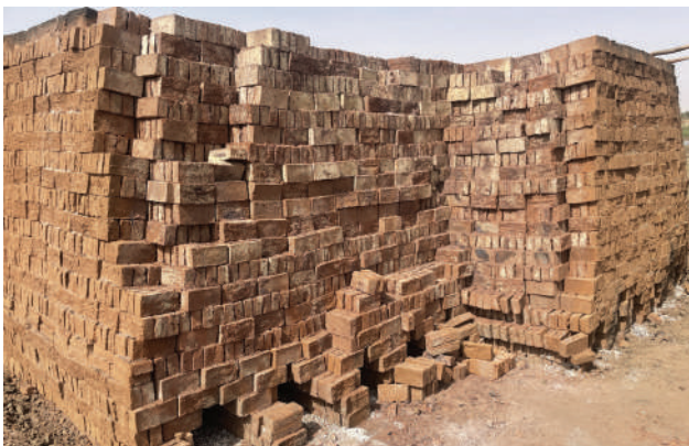
Figure 3: The different red brick qualities inside a kiln in Hillat Koko (Khartoum). © C. Pérez-Houis, April 2022
