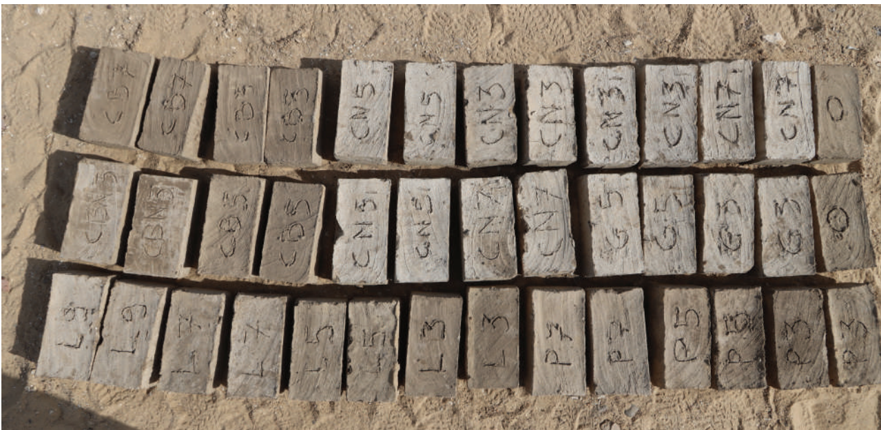
Figure 11: Samples of bricks prepared using a variety of stabilizers and dosages.
