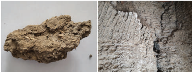
Figure 7: Mortar: sample and arrangement of brick and mortar in masonry vault and wall.
