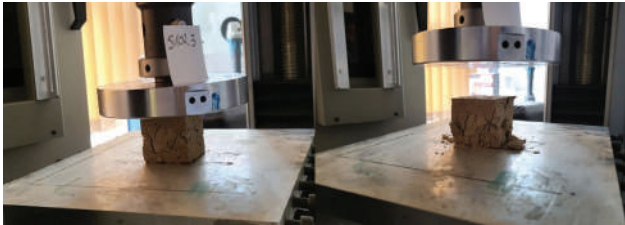
Figure 10: Adobe bricks sample 107_3 before and after compressive strength test.
