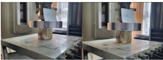
Figure 11: Adobe bricks sample 105_2 before and after compressive strength test.
