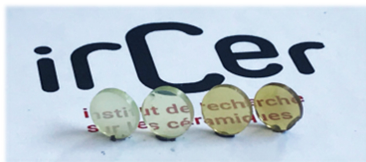
Figure 3. Transparent Ho:Lu 2 O 3 ceramics with various Ho 3+ doping rates (from the left to the right: 0.5 at.%, 1 at.%, 5 at.% and 10 at.%) sintered by SPS at 1400 °C for 15 min under 130 MPa of uniaxial pressure.
