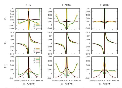
Fig. 4: Line plots of different stress components as a function of the shifted (with respect to the center of the domain along  $x_1$ ) and normalized (with respect to the Burgers vector magnitude b that is equal to lattice constant  $a_0$ ) distance along  $x_1$  passing through the top dislocation at times t = 50, 10000 and 20000. Stress measures associated with KD correspond to  $\sigma'$ .
