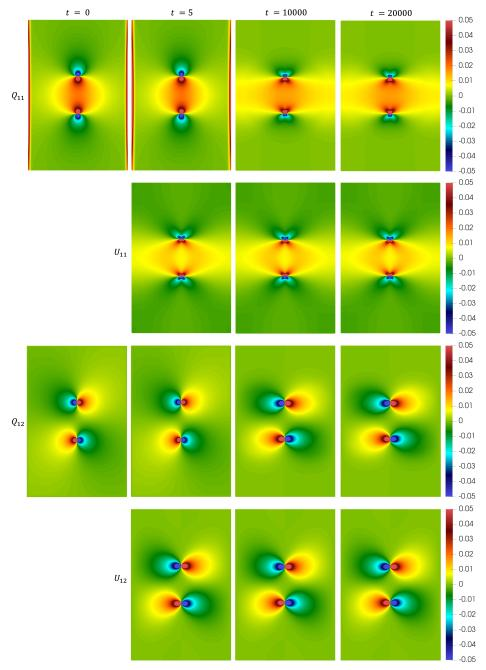
**Fig. 2**: Time evolution of  $Q_{11}$ ,  $U_{11}$ ,  $Q_{22}$  and  $U_{22}$ .  $U_{11}$  and  $U_{22}$  have not been presented at t = 0 due to the instability of dislocation cores in the initial state.
