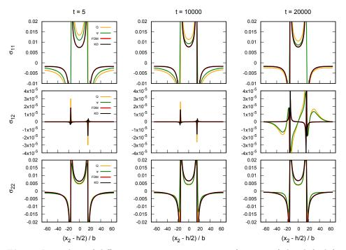
Fig. 3: Line plots of different stress components as a function of the shifted (with respect to the center of the domain along  $x_2$ ) and normalized (with respect to the Burgers vector magnitude b that is equal to lattice constant  $a_0$ ) distance along  $x_2$  passing through the two dislocations at times t = 50, t = 10000 and t = 20000. Stress measures associated with KD correspond to  $\sigma'$ .
