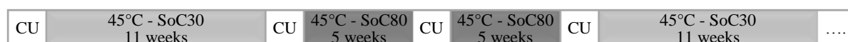
Figure 4 : Planning of the test showing periodicity of Check-Up (CU) and calendar storage at various SoC
