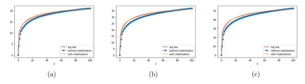
FIGURE 7. Velocity profile with and without stabilization compared with the log-law. (a)  $u^* = 4$ . (b)  $u^* = 7$ . (c)  $u^* = 10$ .
