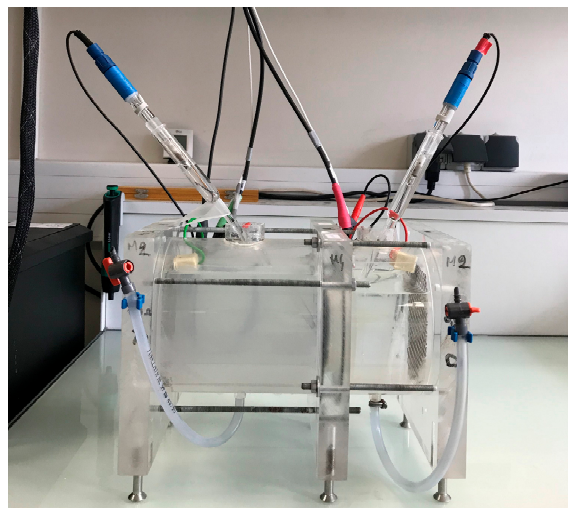
Figure 4. The chloride standard migration test used.
