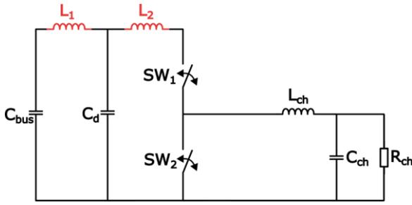
Figure 1: Buck converter with its decoupling capacitor
