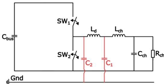
Figure 2: Buck converter with its decoupling inductor
