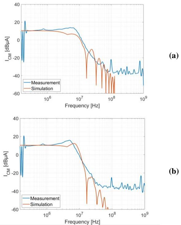
Figure 12: (a) Envelope of CMC spectra without decoupling inductor for measurement and simulation; (b) Envelope of CMC spectra with decoupling inductor for measurement and simulation
