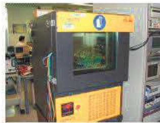
Figure 3. Temperature chamber used for the EMC test
