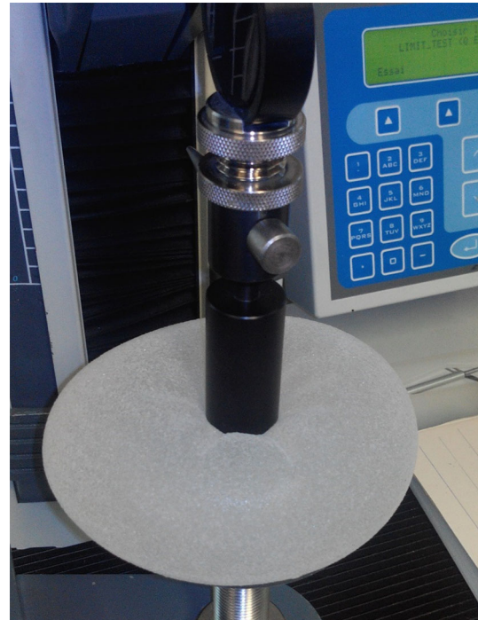
Fig. 1 Implants stiffness test
