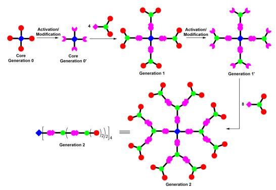
**Scheme 1.** Divergent synthesis of dendrimers. Generation 2 is represented twice: both the full structure, and the corresponding linear representation with parentheses after each branching point.
