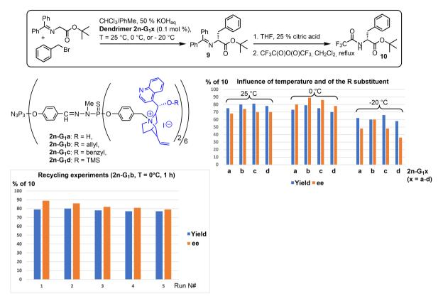
**Scheme 15.** Alkylation of the nitrogen of the quinuclidine of (+)-cinchonine for the grafting to the 1st generation dendrimer. Phase transfer catalyst in the asymmetric alkylation of a glycinate Schiff base with benzyl bromide. Influence of the temperature and the R substituent. Recycling experiments with  $2n-G_1b$ .
