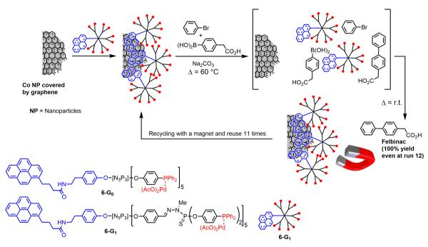
**Scheme 7.** Magnetic cobalt nanoparticles covered by graphene interacting with a pyrene catalytic dendron at room temperature, and used for the synthesis of Felbinac. Recovery using a magnet was carried out 11 times.
