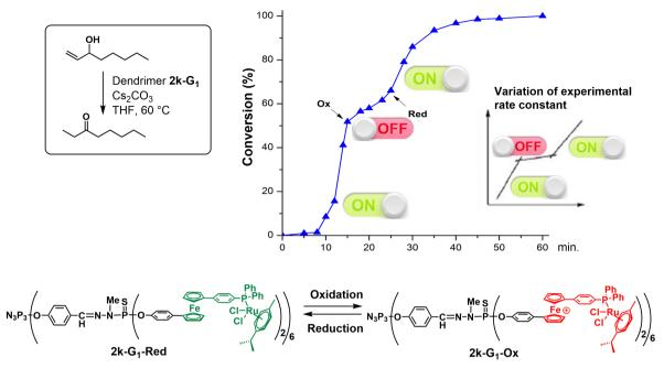
**Scheme 12.** Dendrimer bearing redox switchable phosphines complexing ruthenium, and its use as catalyst in the isomerization of 1-octen-3-ol to 3-octanone. Influence of the oxidation and reduction of the ferrocenes on the catalytic rate.
