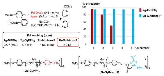
**Scheme 8.** Two types of dendrimers suitable for the complexation of palladium, and used in Suzuki couplings. Recycling was only efficient with the dendrimer bearing the thiazolyl phosphine complexes, thanks to undetectable palladium leaching.
