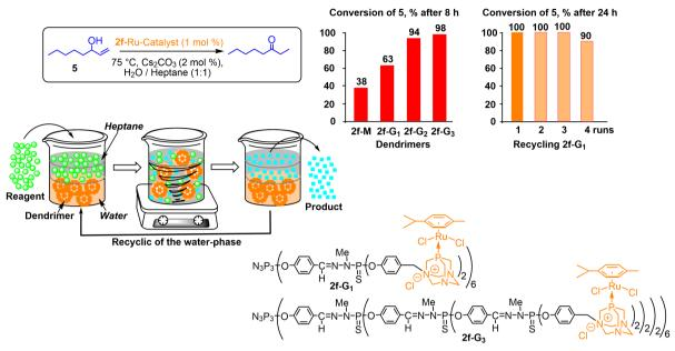
**Scheme 6.** Water-soluble dendrimers used in catalyzed biphasic isomerization of allylic alcohols to ketones. Positive dendritic effect, and recycling of **2f-G<sub>1</sub>** by phase separation.
