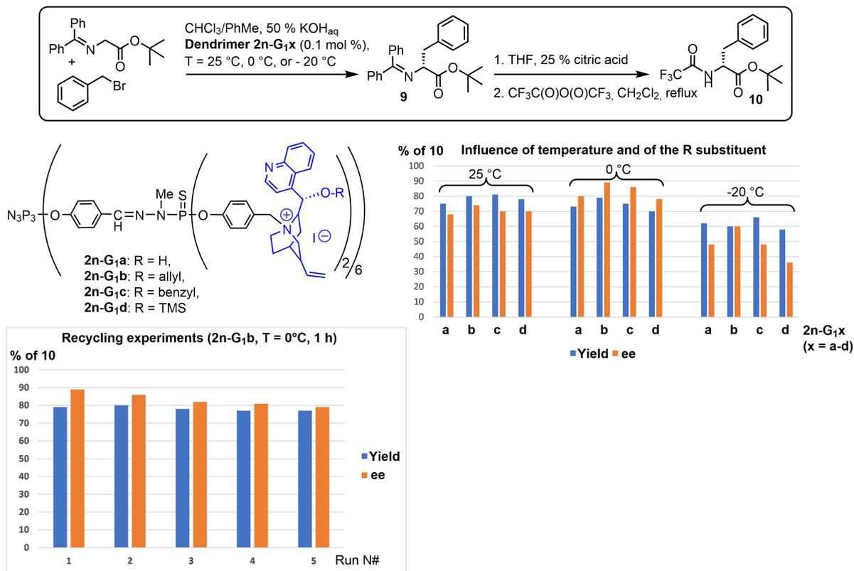
**Scheme 15.** Alkylation of the nitrogen of the quinuclidine of (+)-cinchonine for the grafting to the 1st generation dendrimer. Phase transfer catalyst in the asymmetric alkylation of a glycinate Schiff base with benzyl bromide. Influence of the temperature and the R substituent. Recycling experiments with **2n-G<sub>1</sub>b**.
