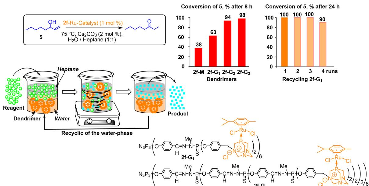
**Scheme 6.** Water-soluble dendrimers used in catalyzed biphasic isomerization of allylic alcohols to ketones. Positive dendritic effect, and recycling of **2f-G<sub>1</sub>** by phase separation.
