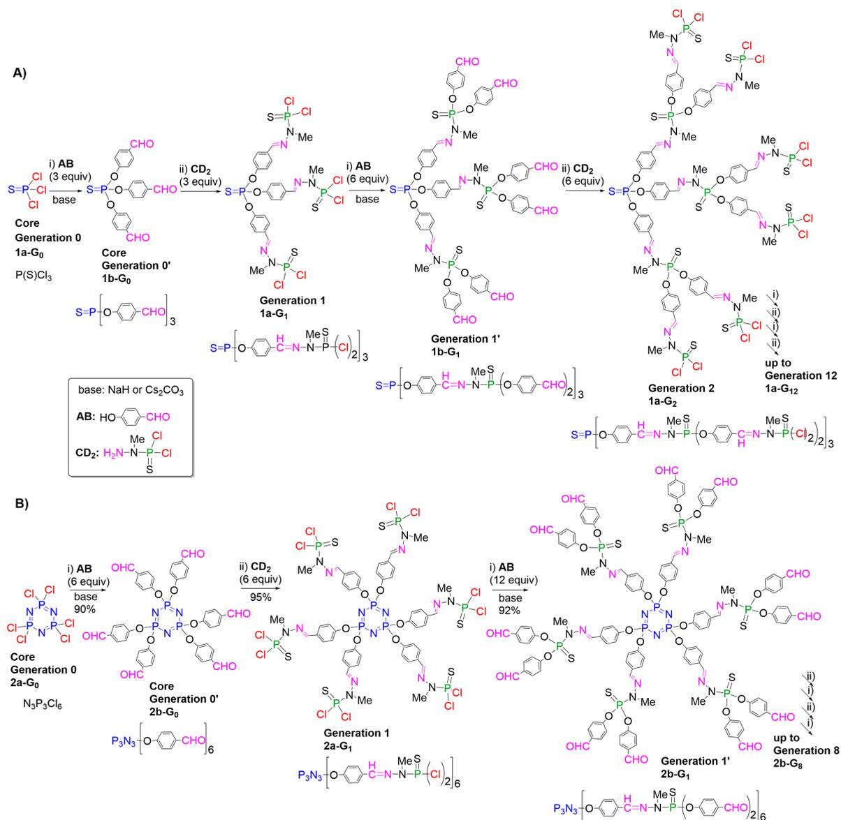
**Scheme 2.** Synthesis of polyphosphorhydrazone dendrimers, starting from either P(S)Cl<sub>3</sub> (A) or N<sub>3</sub>P<sub>3</sub>Cl<sub>6</sub> (B) as core.
