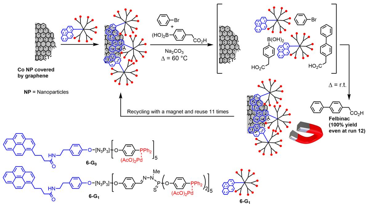
**Scheme 7.** Magnetic cobalt nanoparticles covered by graphene interacting with a pyrene catalytic dendron at room temperature, and used for the synthesis of Felbinac. Recovery using a magnet was carried out 11 times.
