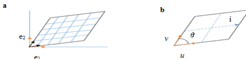
Fig. 1. Anisotropic network - local and global basis Sossoe et al. (2015) : (a) Anisotropic network with a mesh of 2D cells in an orthonormal basis ( e_1, e_2 ) and a local basis ( u, v ); (b) Zoom on a 2D elementary cell.
