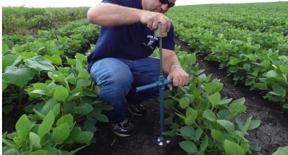
Figure 23: Gravimetric sampling, where a surface soil core of known volume is collected at multiple depths for comparison to aircraft and satellite products.
