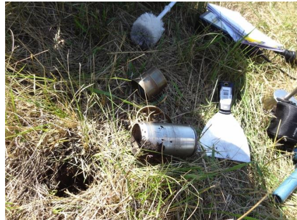
Figure 23: Gravimetric sampling, where a surface soil core of known volume is collected at multiple depths for comparison to aircraft and satellite products.
