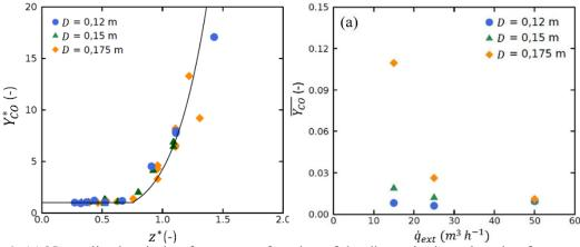
Figure 4: (a) Normalised emission factors as a function of the dimensionless elevation for tests carried out at 50 m<sup>3</sup> h<sup>-1</sup>, (b) CO emission versus the ventilation flow rate for 3 pool diameters and at elevation  $z_b/H=0.41$
