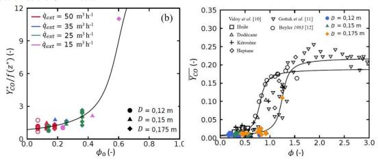
Figure 5: Emission factors as a function of the equivalence ratio for the tests of the present study but also Valoy et al. [10], Gottuk et al. [11] and Beyler et al. [12]. Laws of evolution proposed by Gottuk et al. [9].
