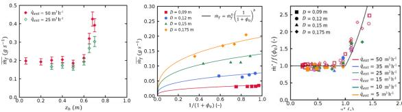
Figure 3: (a) Global MLR as a function of the elevation for two ventilation flow rates (D=0.175 m) (b), Global MLR as a function of the ventilation factor for four pool diameters (z<sub>b</sub>/H=0.41) (c) Dimensionless MLR as a function of the dimensionless elevation.
