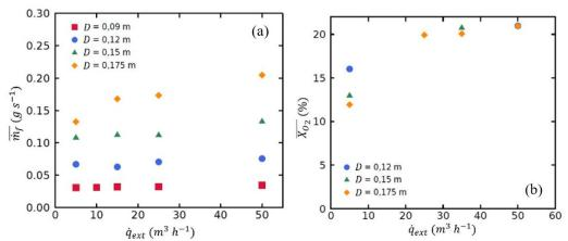
Figure 2: Global MLR (a) and mean oxygen concentration near the fuel pan (b) as a function of the ventilation flow rate for the different pan diameters (fire elevation z<sub>b</sub>/H=0,41).
