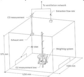
Figure 1: NYX reduced-scale experimental device and measurements.
