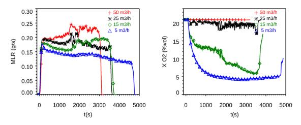
Figure 2: Effect of ventilation flow rate on the time variation of the MLR (a) and oxygen concentration at 0.55 from the ground (b) (pool fire of D=0.175 m and elevation  $z_b/H = 0.41$ ).
