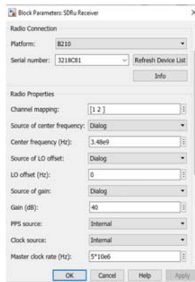
Figure 7: Programming USRP via Simulink
