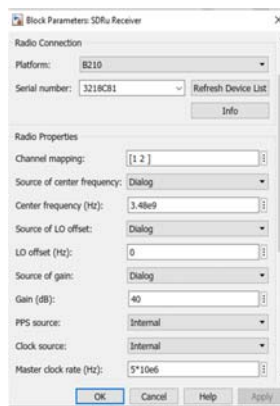
Figure 7: Programming USRP via Simulink
