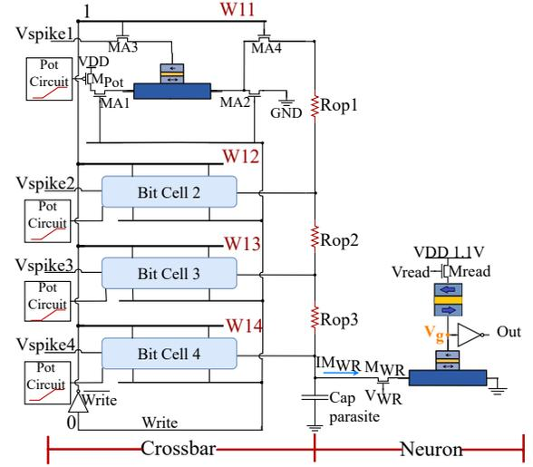
Fig. 5: Crossbar of the SNN under analysis with possible open locations.
