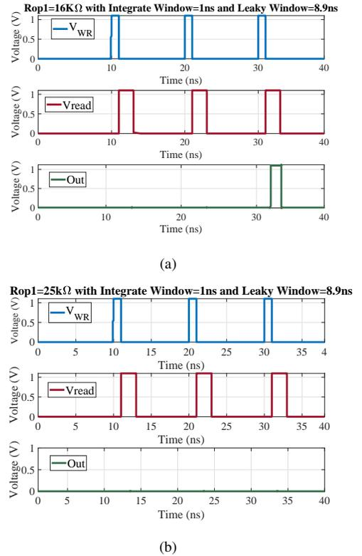
Fig. 12: Fault analysis modifying the Leaky Window.
