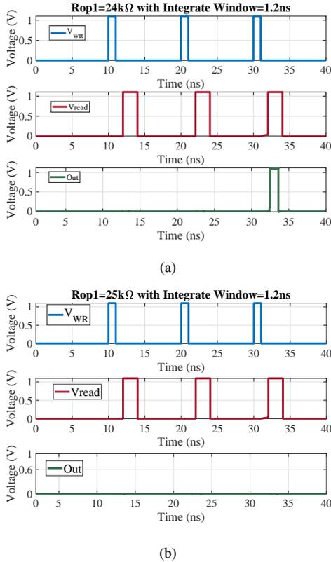
Fig. 11: Fault analysis modifying the Integrate Window.
