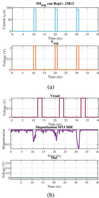
Fig. 8: Behavior of the crossbar of the SNN with open  $R_{op1}$  with a resistance of  $23\text{K}\Omega$ .
