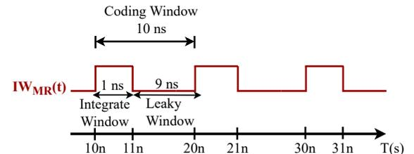
Fig. 6: Timing conditions of the Integrate Window and Leaky Window of the neuron.
